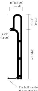
The hull standoff is located on the 3rd step down 36" (92 cm) below the brackets for all ladders up to 5 steps long.
