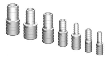
Tru-Design Reducers are moulded from a glass reinforced nylon composite. High strength, high-modulus glass fibres impregnated into the nylon provides dramatic strength, stiffness, toughness, and dimensional stability.
