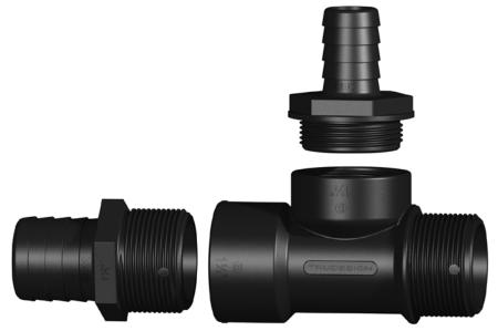
The **TRUDESIGN®** T-Piece Connector is commonly used in glycol/antifreeze flush-through systems when preparing for winterization, or, in fresh water engine flush systems. By adding a plug to the female end, the T-Piece Connector can function as an inspection port for looking through to, or clearing the internals of a Ball Valve.
