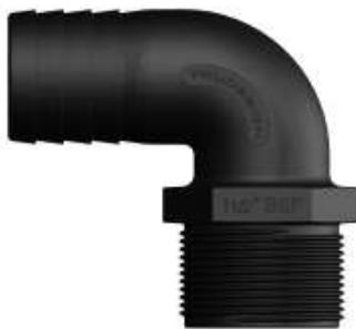
TruDesign Tails are moulded from a glass reinforced nylon composite. High strength, high-modulus glass fibres impregnated into the nylon provides dramatic strength, stiffness, toughness, and dimensional stability. TruDesign Tails eliminate the corrosion and electrical bonding problems associated with metallic fittings. The Tails are designed for twin hose clamps, and to not crush under high load conditions.
